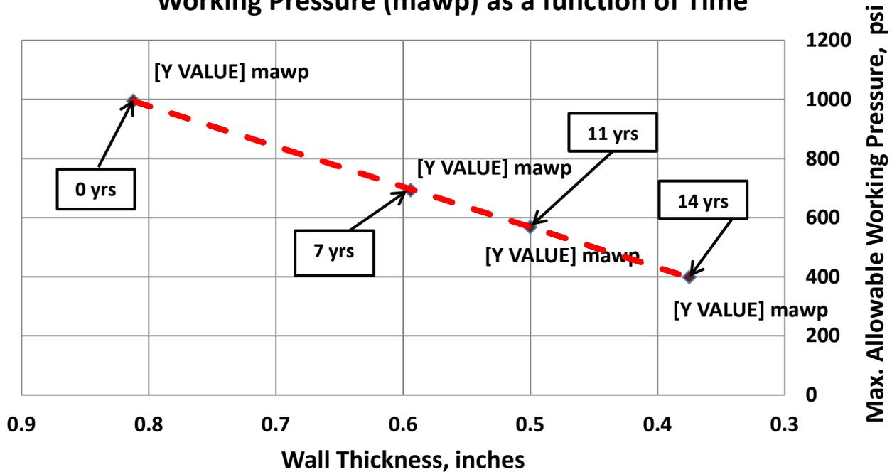
Figure 2 is a plot of Maximum Allowable Working Pressure (mawp) for schedule 60, 20 inch outside diameter, seamless carbon steel pipe.<sup>19</sup> This is the pipe that was installed at the Straits of Mackinac in 1953.
